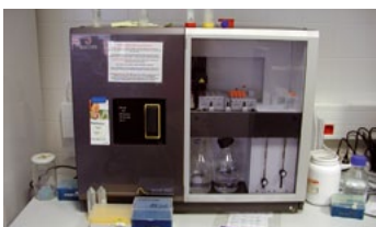
Photo 3 Instrumentation for SPR (surface plasmon resonance)
