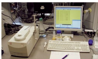
Photo 2 Instrumentation for ITC (isothermal titration calorimetry)
