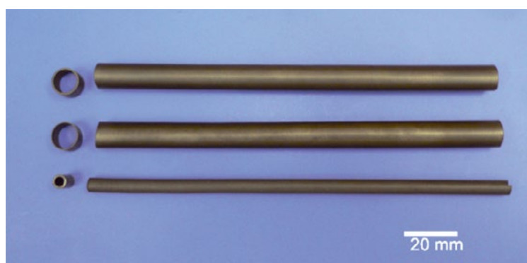
Photo 1 Electroceramics – Oxygen tubular membranes, material: La-Ca-Fe-Co perovskite
