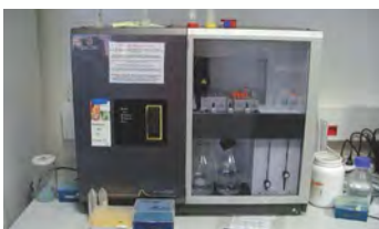
Photo 3 Instrumentation for SPR (surface plasmon resonance)
