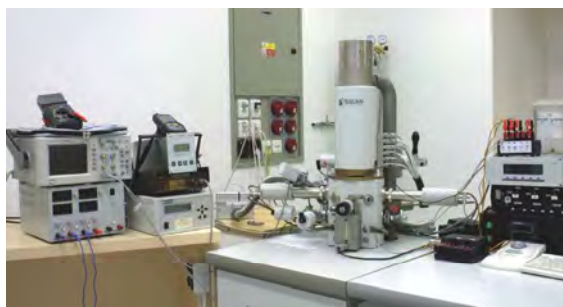
Fig 1 Environmental scanning electron microscopy AQUAEM II
