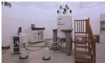
Photo 1 600 MHz NMR spectrometer Bruker AVANCE
