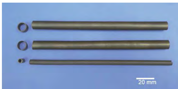
Photo 1 Electroceramics – Oxygen tubular membranes, material: La-Ca-Fe-Co perovskite
