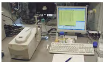
Photo 2 Instrumentation for ITC (isothermal titration calorimetry)
