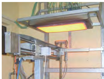
Photo 1 HTC measurement: Continuous casting, secondary cooling
